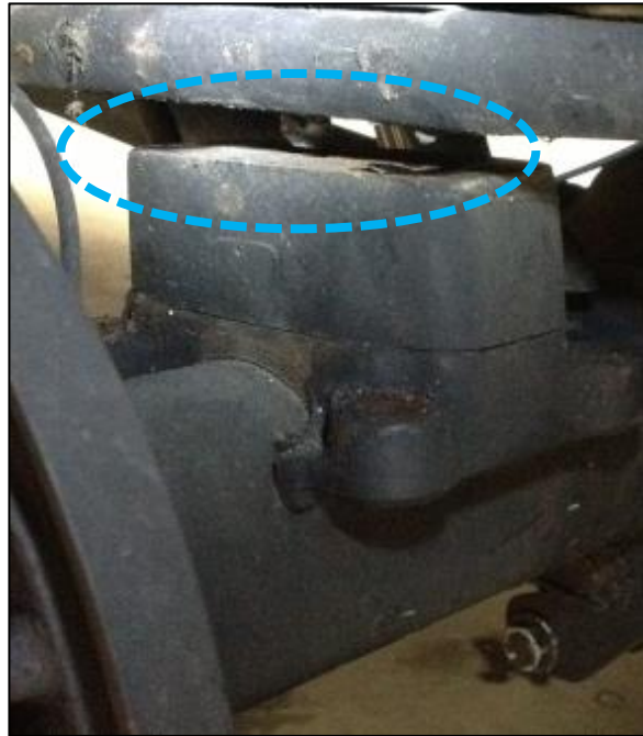
Original position of extended leaf spring spacer
